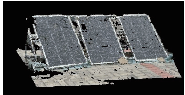
图 6 光伏发电板三维静态模型重建结果 Fig. 6 Results of 3D static model reconstruction for photovoltaic panels
